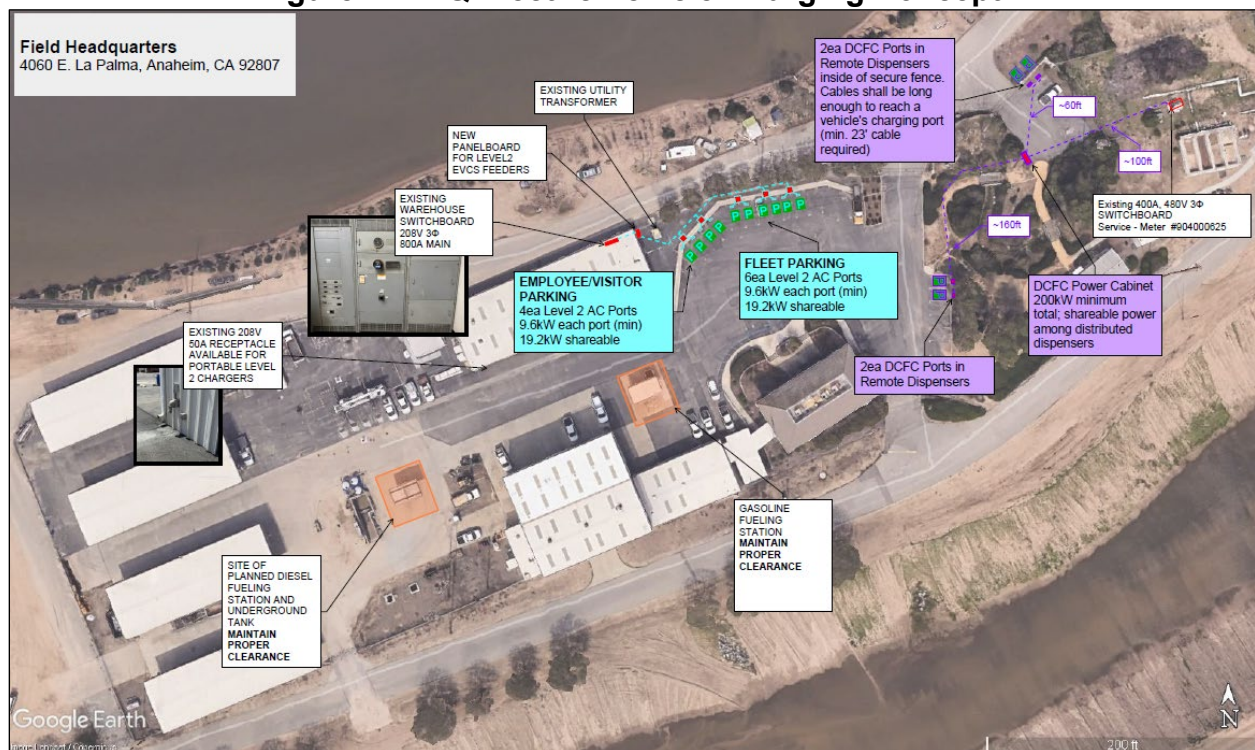
Figure 1: FHQ Electric Vehicle Charging Concept
