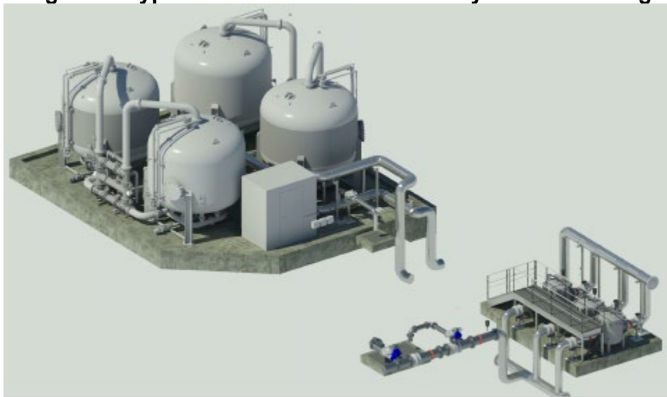
Figure 2: Typical Four-Vessel Treatment System Rendering
