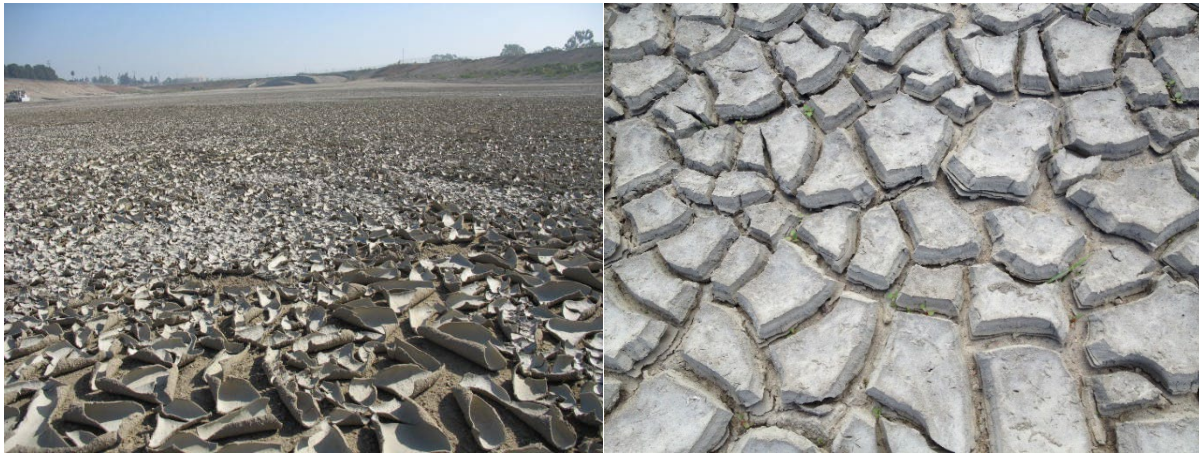
Figure 22: Clogging Layer in a Recharge Basin
