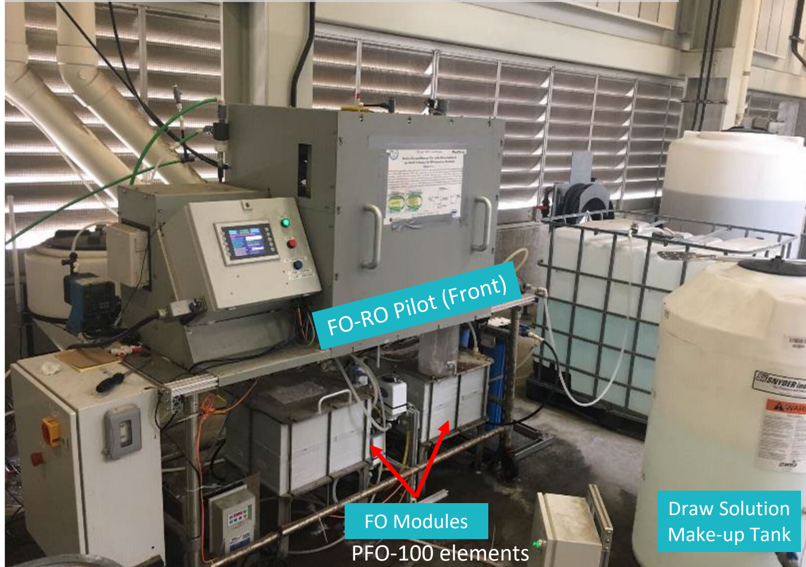
1-gpm FO-RO Pilot at OCWD GWRS AWPf RO Building
