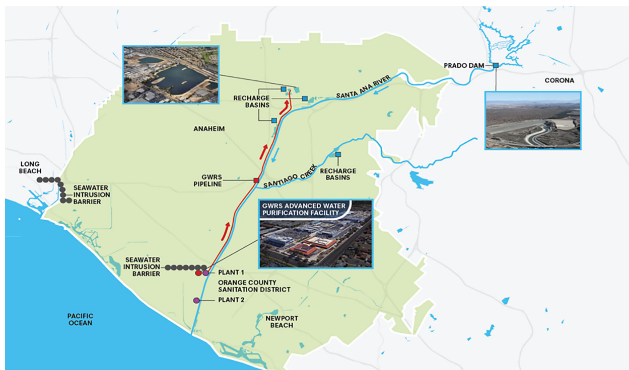
FIGURE 1. The Groundwater Replenishment System. Source: 2017 GWRs Annual Report. Map of the Groundwater Replenishment System, including locations of the infiltration basins. Orange County Water District. Groundwater Replenishment System 2017 Annual Report . Available at https://www.ocwd.com/media/6822/2017-gwrs-annual-report.pdf .
