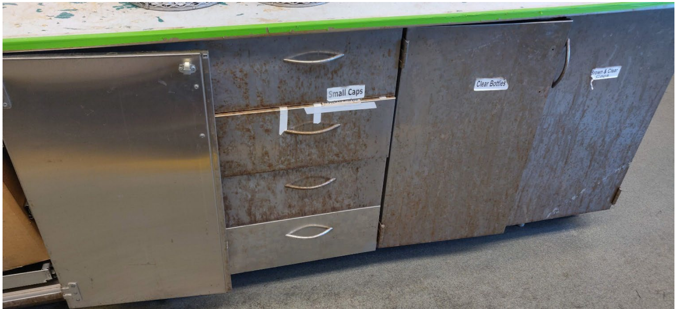
Photo 3: Comparison of external damage of cabinetry versus internal, unexposed stainless-steel
