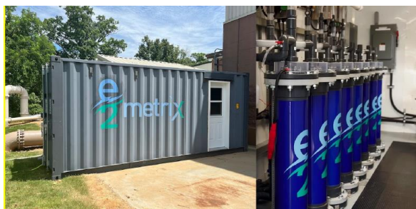
Figure 4. ECOTHOR-AOP integrated solution of E2Mmetrix-OVIVO showing 20 ft container housing the pilots on the left and electrodes on the right.
