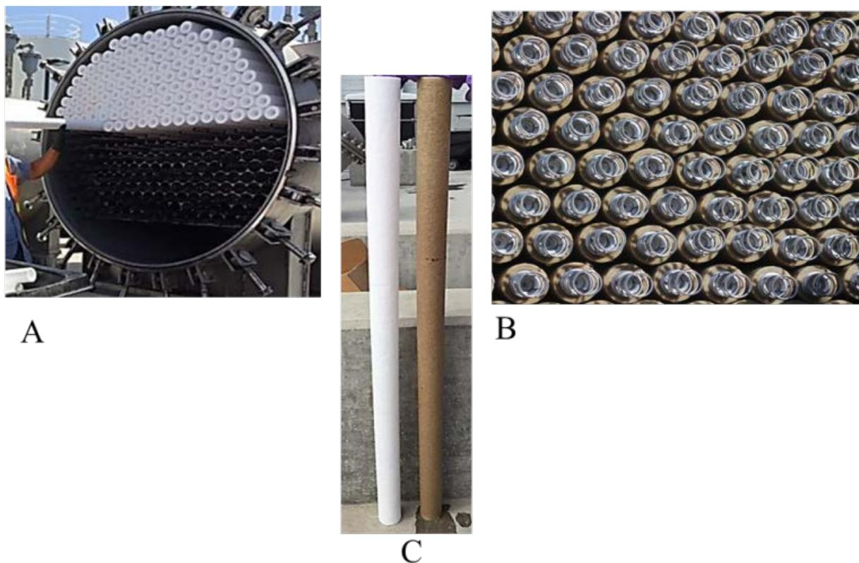
**Figure 1.** CF replacement: A) new CFs, B) used CFs ready for replacement, and C) comparison of new (white) CF and fouled (brown) CF.
