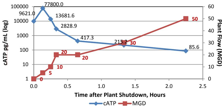
**Figure 5.** CF effluent cATP concentrations after a 7.5-hr. shutdown. cATP was measured at intervals during the plant start up, 0 – 50 mgd.
