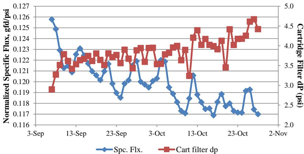
**Figure 3.** CF differential pressure and RO membrane performance as indicated by normalized specific flux (dP = differential pressure; gfd = gallons per square foot per day; psi = pounds per square inch),
