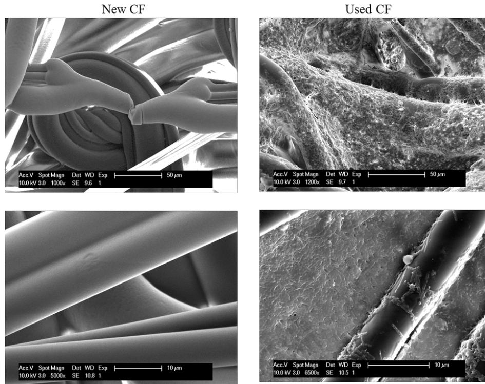
**Figure 2.** SEM of a new and used cartridge filters.
