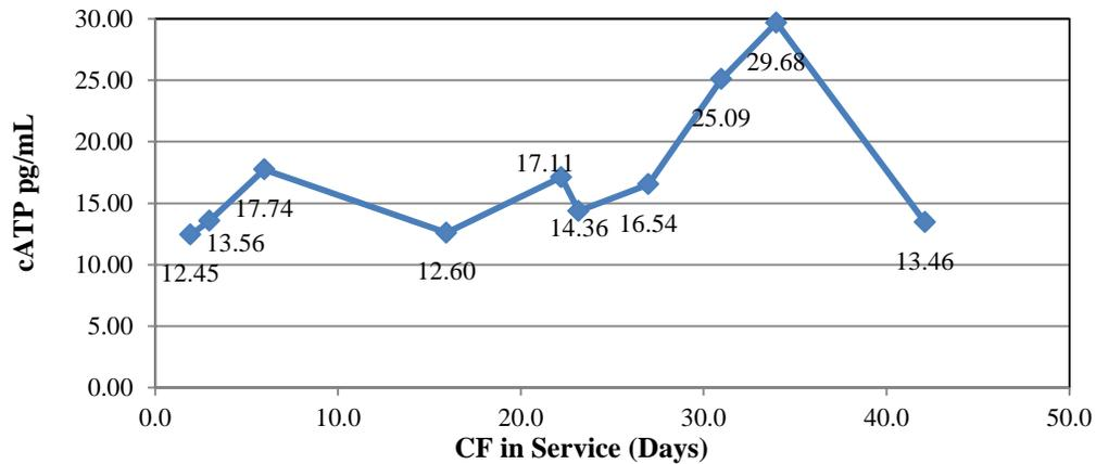
**Figure 6.** Typical profile of CF effluent cATP concentrations after CF replacement at Day 0.
