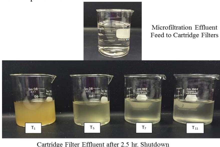
**Figure 8.** Visual difference between CF influent and CF effluent after 2.5-hr plant shutdown. CF effluent samples were collected at 1, 5, 7 and 11 minutes during CF flush to waste procedure.
