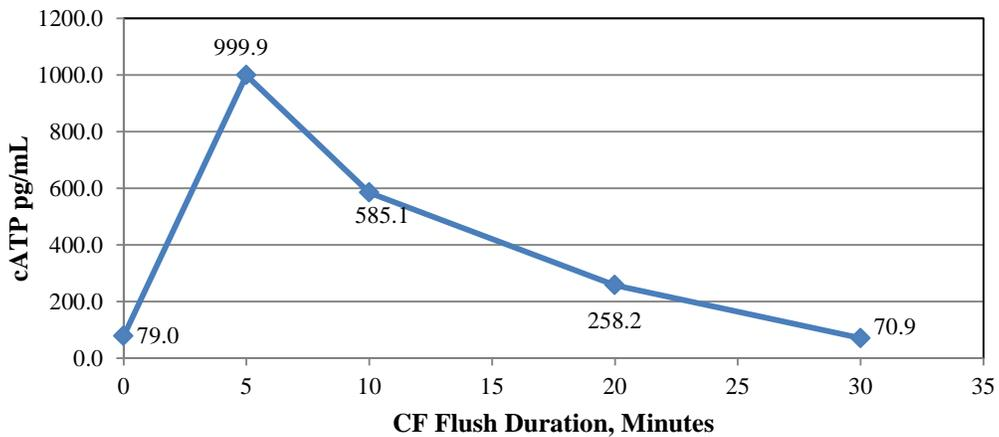
**Figure 7.** CF effluent cATP concentrations collected during flush to waste procedure after a 5-hr. plant shutdown.
