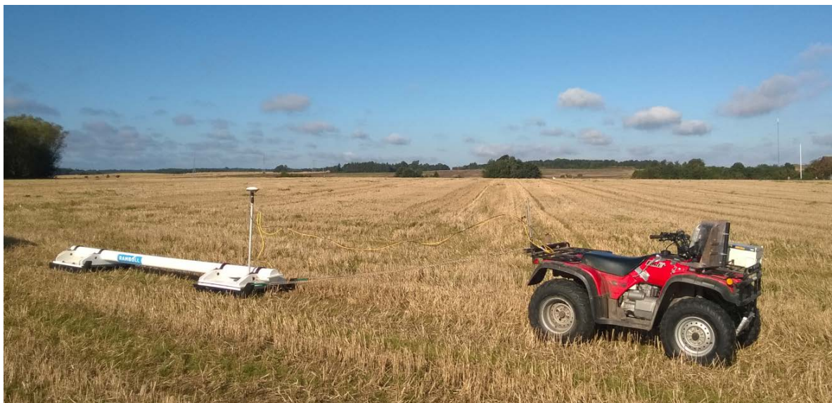
Figure 3 The DualEM421s sensor pulled behind an ATV
