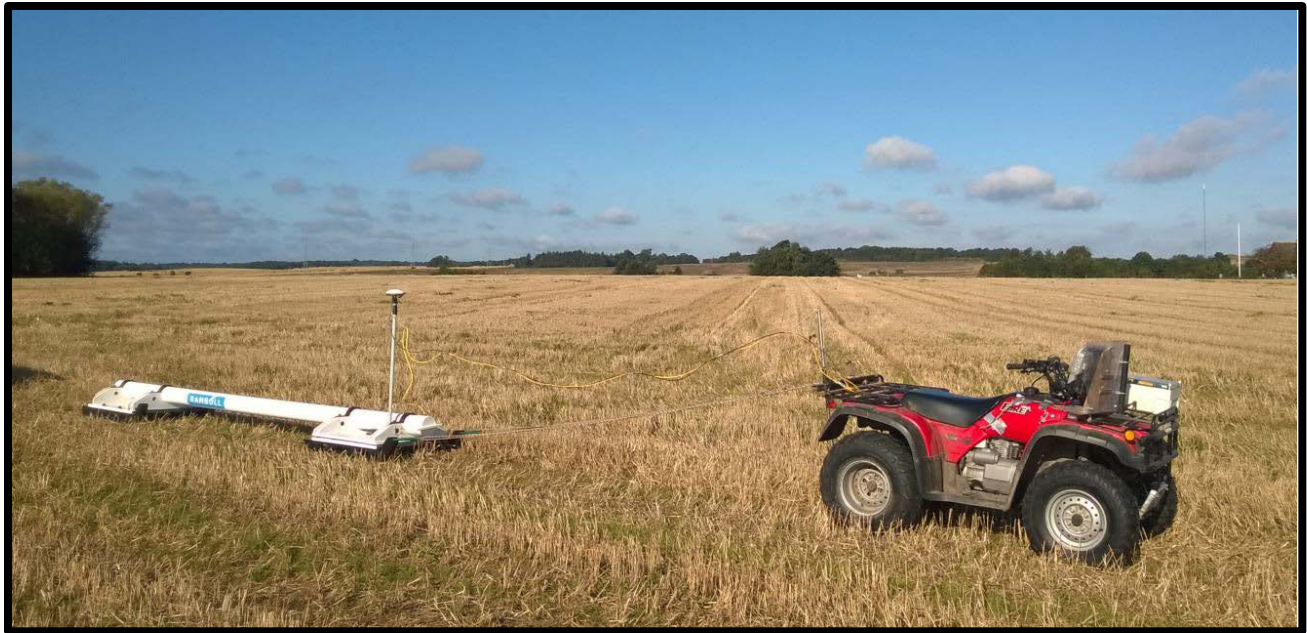
Figure 2 DualEM421s sensor pulled behind an ATV
