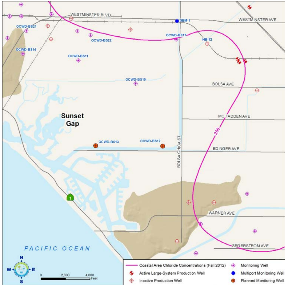
Figure 7-7: Sunset Gap Monitoring and Production Wells with Chloride Concentration Contour
